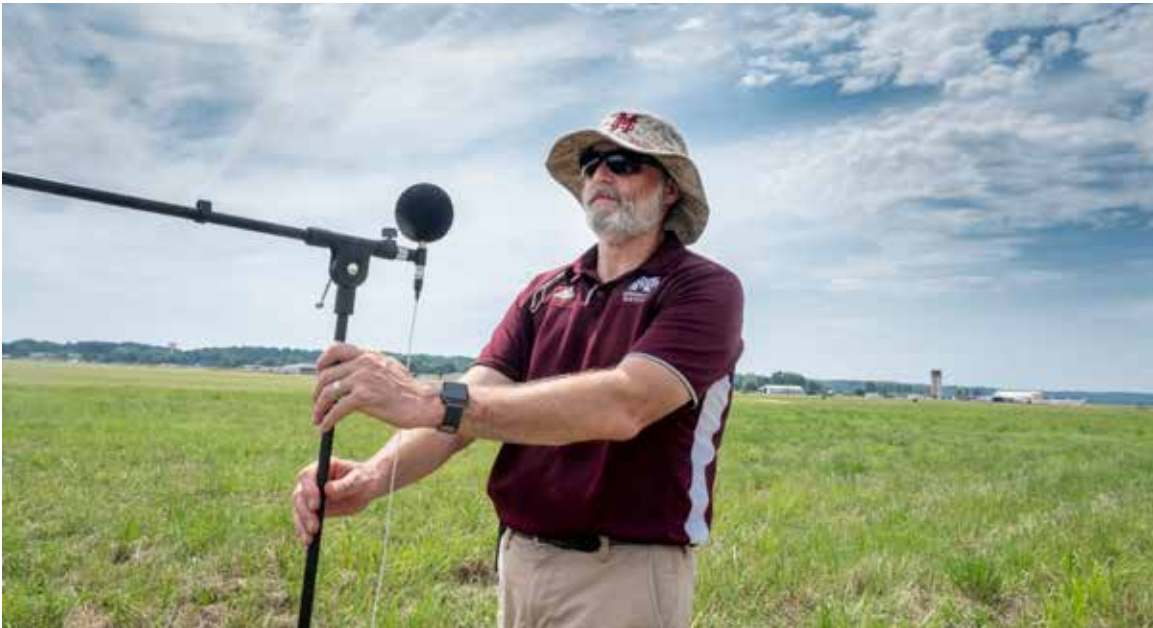
Tom Brooks adjusts one in an array of microphones at Greenwood-LeFlore Airport in preparation for acoustic measurements of an unmanned aircraft system flight.
